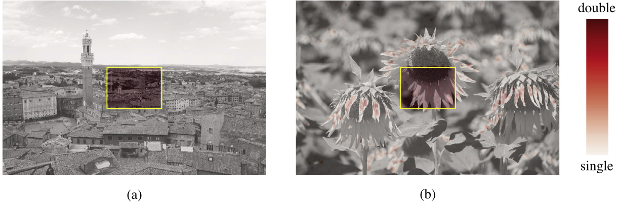
Fig. 10. A-DJPEG (a) and NA-DJPEG (b) localization example of a compressed central region with QF2 = 95 and QF1 = 80. C_{hist} is used for the aligned case while C_{noise} for the non aligned case. Actual forged region lies inside the yellow rectangle.
